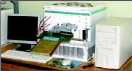
**WS-1 (Workstation 1)** is designed for diagnostics and fault finding up to the element level (a group of elements) of digital and digital-to-analog LRUs based on TTL, CMOS or mixed TTL-CMOS logic as well as LRUs having analog elements with signal levels over the range from
