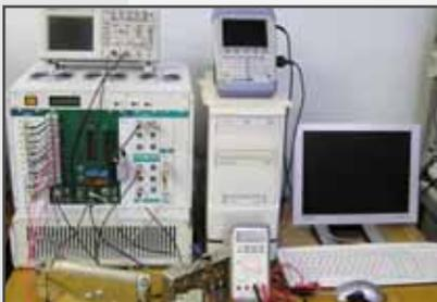
**WS-2 (Workstation 2)** is the PC-based measuring-diagnostic complex, which is designed to diagnose and measure the high-frequency LRU parameters.
